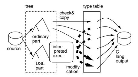
Figure 9: The structure of o3 compiler
