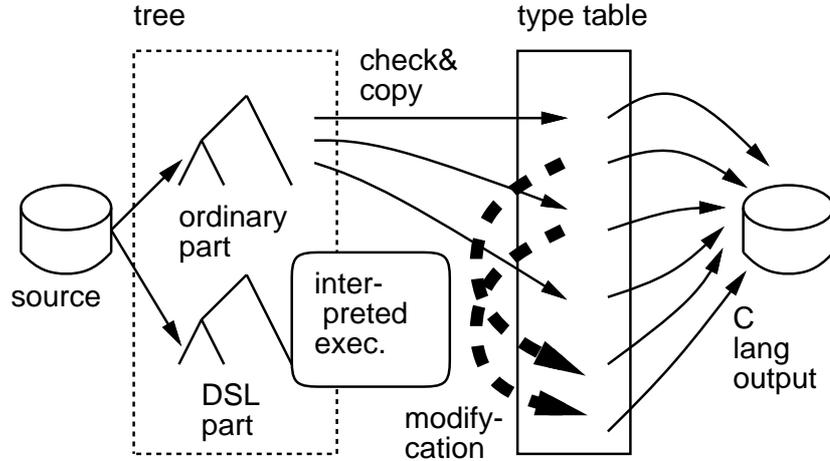
Figure 9: The structure of o3 compiler
